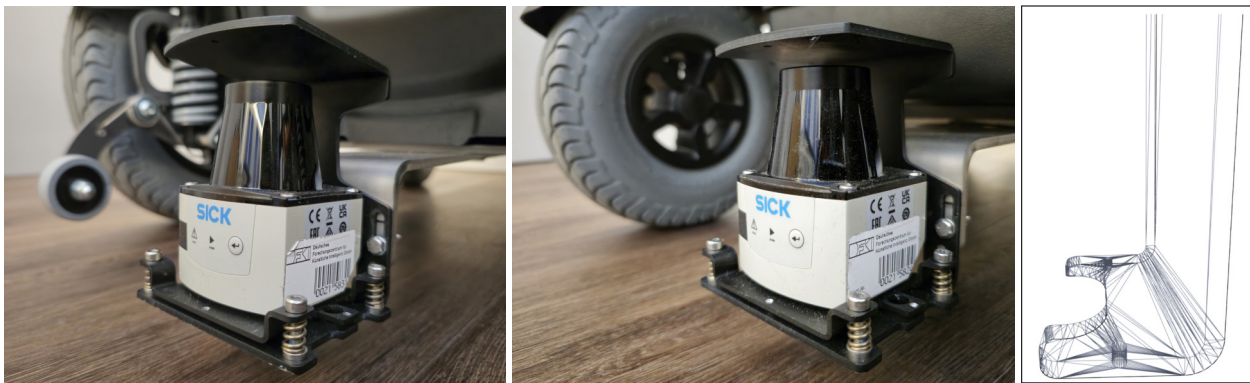
Figure 4: From left to right: front laser scanner, rear laser scanner, and CAD-rendering of LiDAR-mount designed by DFKI. Both laserscanners are protected by cages that allow for accurate alignment of the sensor.
