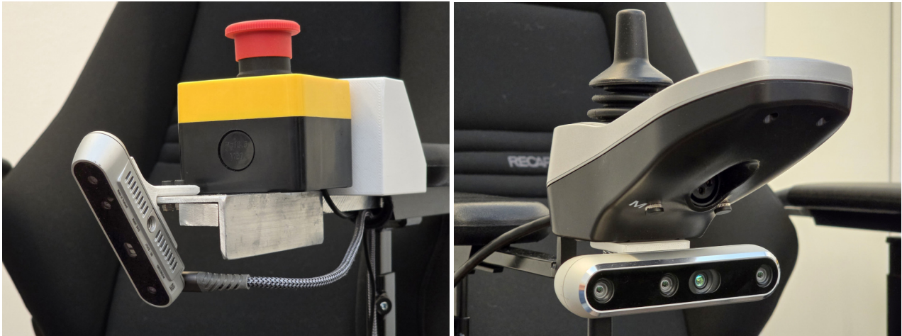
Figure 5: Vertically and horizontally RGBD-cameras mounted on the left and right armrest respectively.
